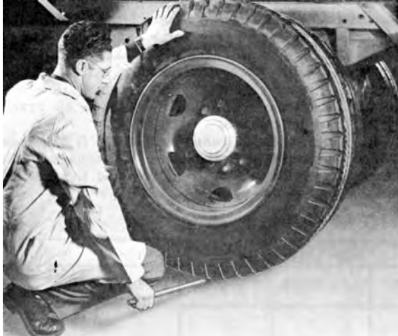
Figure 3-6 Checking for Loose Wheel Bearings
