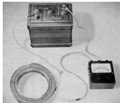
Figure 3-15 Testing Amperage Capacity of Magnet
