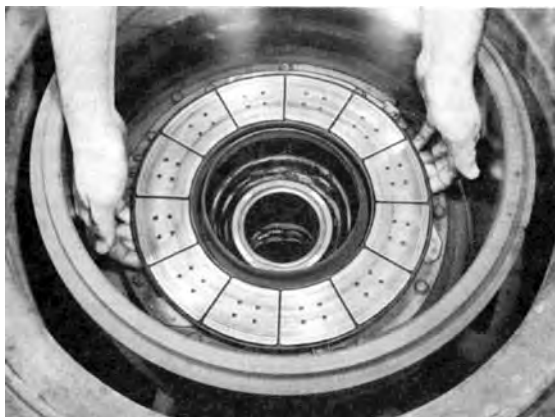
Figure 2-15 Positioning Armature Disc
