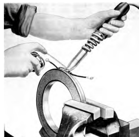
Figure 3-18 Soldering Magnet Lead Wires
