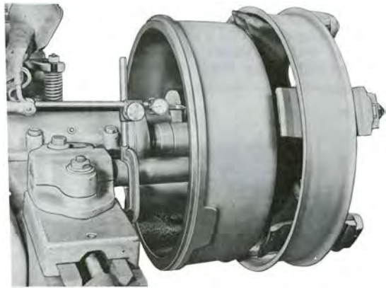
Figure 2-2 Checking Drum on Lathe
