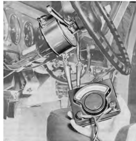
Figure 3-2 Connecting Ammeter to Controller and Brake Wire
