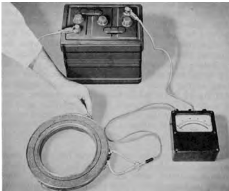
Figure 3-16 Testing Magnet for Ground
