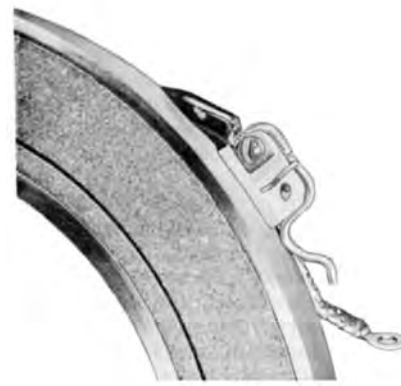
Figure 3-20 Installing Leads in Ceramic Block
