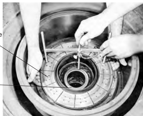
Figure 2-16 Using Depression Gauge—Step 3
