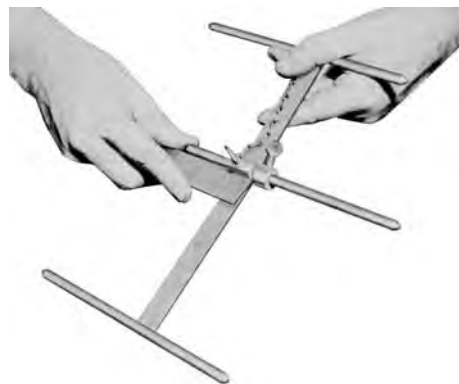
Figure 2-17 Measuring Armature Depression
