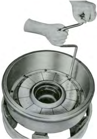
Figure 2-11 Bolt Armature Inside of Drum
