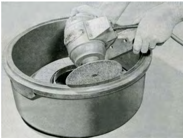
Figure 3-10 Removing Ridge on Drum
