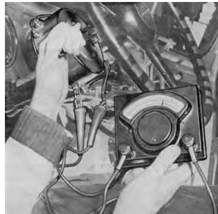
Figure 3-3 Checking Circuit Current
