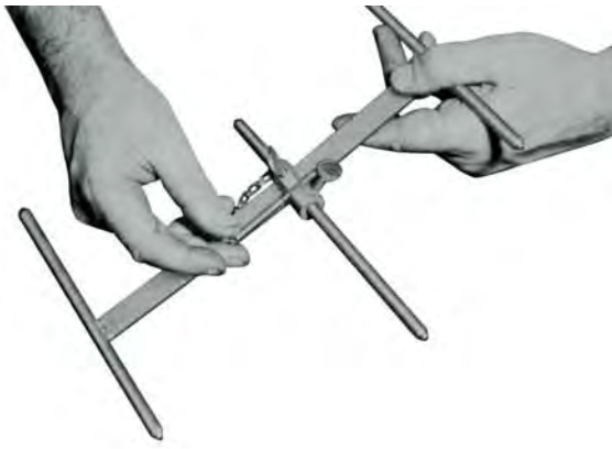
Figure 2-18 Using GO-NO-GO Gauge
