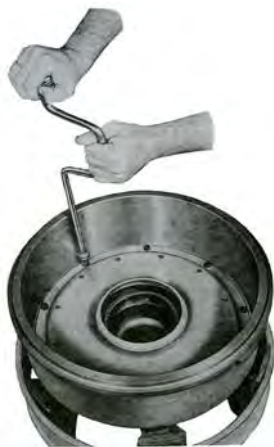
Figure 2-4 Bolting Armature Adapter to Drum
